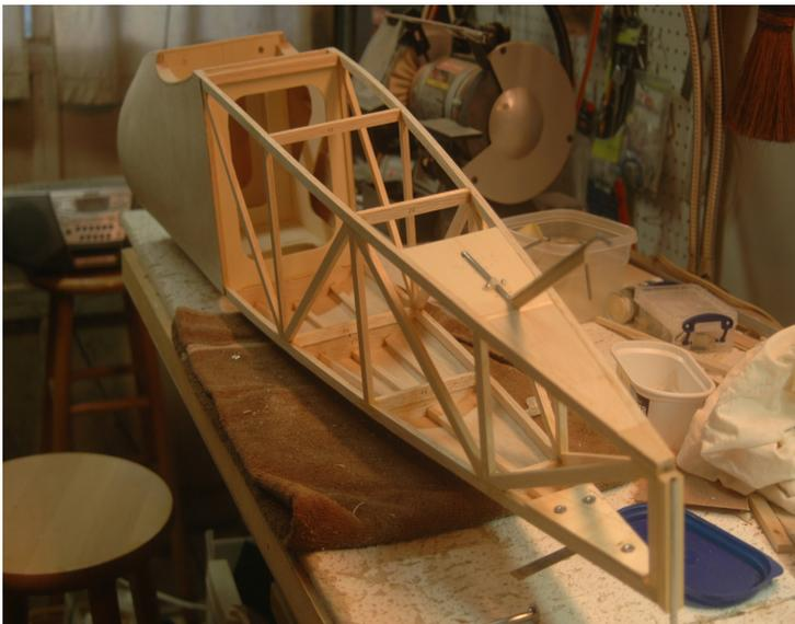
The Nieuport getting its tail skid. This is just the beginning of the process. On the first one, the tail skid built per plans was very easily knocked loose due to lateral pressure on it when the plane was turned on the runway. The whole structure is quite large so I beefed that one up with plywood side supports and a quarter square hardwood rail on both sides of the side supports for a larger footprint on the fuselage.
