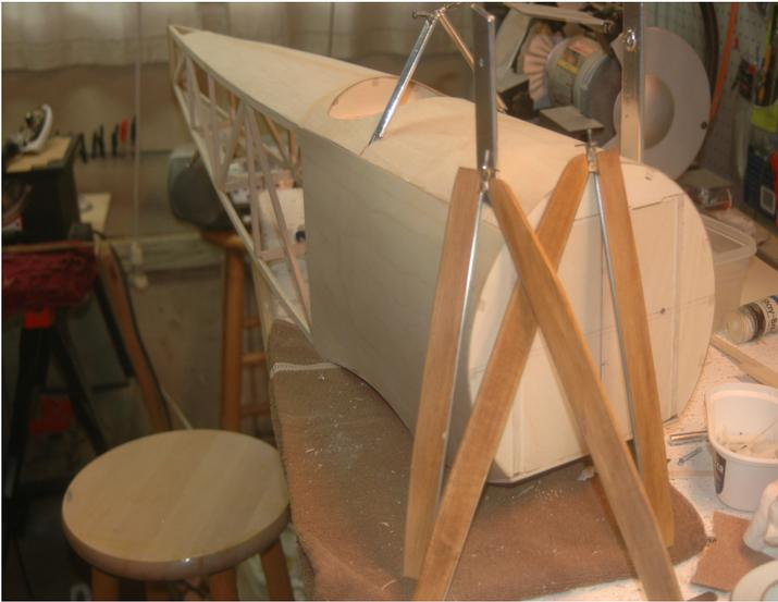
The wing struts are stained and I plan to varnish them next. The cabane struts are covered with aluminum tape that I got at Lowes.
