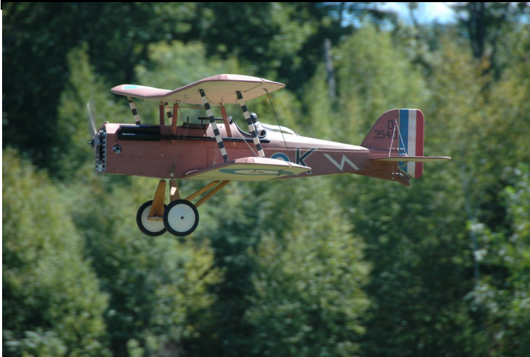
Ron Prestin's beautiful 1/4 scale SE-5. This plane was finished just in time for the Jamboree. He built it from a Fun Aero kit and powered it with a Cheetah 42. It's covered with Solartex and painted with latex color matched to a Replicraft PC-12 chip. Ron and his friend Bob Allen kept it quite busy during the weekend.
