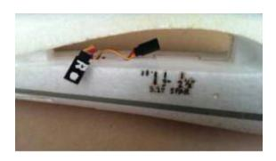
**Stab decalage** -- the out-of-the-box stab decalage is way too positive (possibly to offset the extreme nose heavy balance just described). You must change it to compensate for the revised CG. Raise the leading edge of the stab by about 3/32". To do so, remove the plastic rudder doublers, carve out a bit of rudder foam with an Exacto knife and raise the leading edge. Backfill the void
