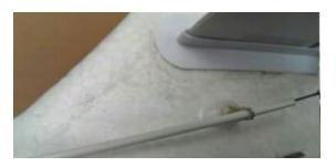
Rudder Elevator Pushrod Clevises -- the stock Radian pushrod-horn screw clevises are junk. Sooner or later you will over-tighten and twist off the thumb cap. Then you are stuck! Replace both rudder and elevator screws with nylon or metal clevises and threaded brass pushrod ends. Solder or epoxy the ends to the pushrods.
