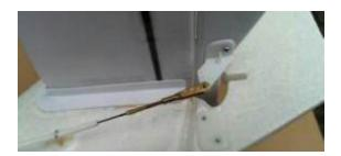
Ventilation Grill -- the grass is usually wet in the early morning at the Wallkill field. Tape over the RX/servo hatch/grill otherwise you will be draining water out of your RX pack. Don't be concerned about motor ventilation; you are a glider using the motor for 30 seconds to get to altitude - not a power plane doing acrobats for 5 minutes.
