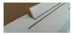
Some on-line videos show how to make silicone hinges. For the Radian, it's not worth the effort or additional weight. If you feel like it, you can cover the gap between with a thin plastic strip. You can bond two strips of Book Tape - glue-side to glue-side - to make a thin film cover.
