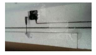
Use the same Dremel Tool and bit to route servo pockets and wire conduits. The wing is plenty thick and you can bury the servos flush with the bottom chord.
