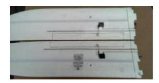
Start with a standard Radian wing or get a wing/spar replacement kit (EFL4702). Inspect the trailing edge and mark off the longest stretch that is straight. Start about 11/2" from the root plug-in area and measure towards the tip for about 16". Make your flaps about 11/2" wide. Mark and cut them free with a single edged razor blade.
