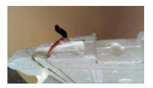
The flap servo location has added weight aft of the CG so you will have to rebalance your Radian to get the CG described earlier. You can usually rebalance simply by moving your battery pack forward. Add a foam block behind the pack to keep it from sliding aft on launch.
